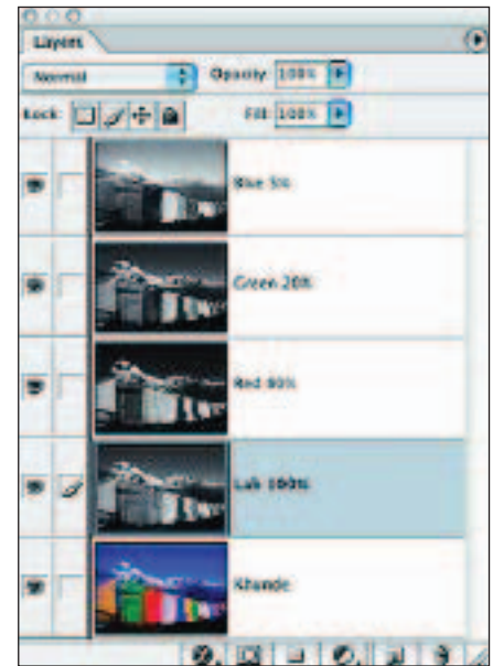
FIGURE 4-27. LAYERS PALETTE, CHANNELS AS LAYERS. The position of the original color image layer, Lightness channel, and RGB channels is shown. Each of the color channels is a grayscale image with layer opacity adjusted as indicated in the figure and text.
